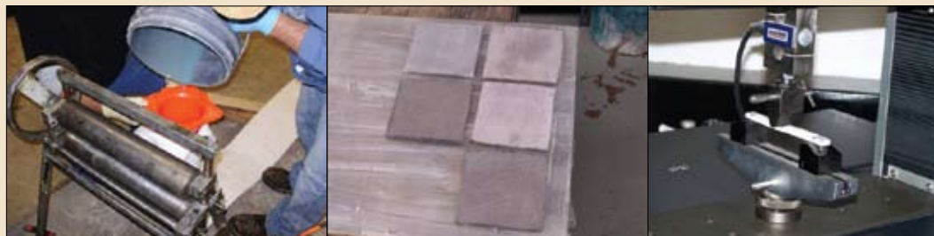
Fig 1. Roller system (left), impregnated panels (middle), and mechanical testing (right)
