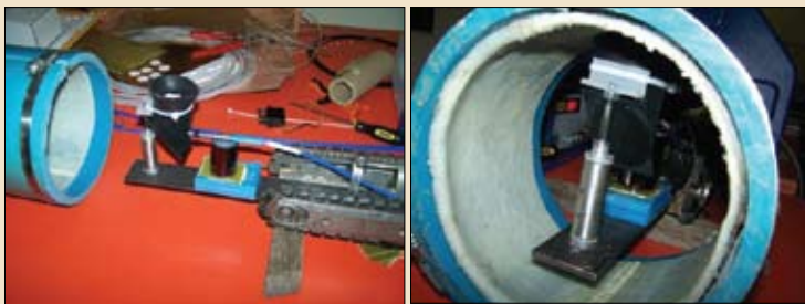
Fig 3 A prototype of the LinerRite sensor mounted on a robotic platform during laboratory tests
