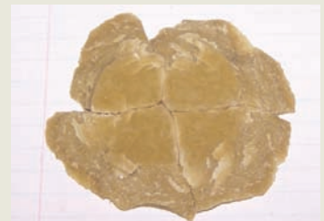
Fig 9. Puncture hole and fragments - polyurethane
