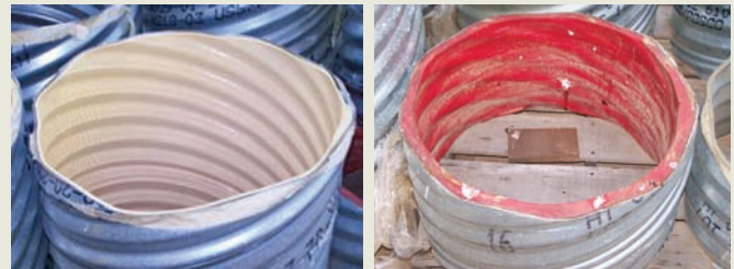
Fig 2. Twenty-four inch corrugated metal pipes coated with different formulations of polyurea await testing at the Trenchless Technology Center
