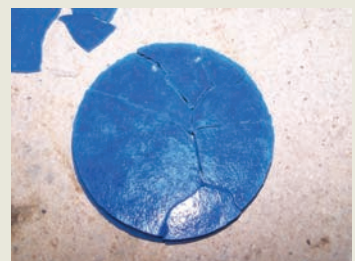
Fig 10. Puncture hole and fragments - polyurea
