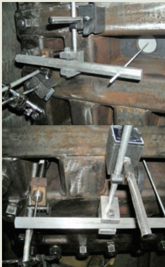
Fig 7. LVDT installed at panel opening (top: side view, bottom: top view).
