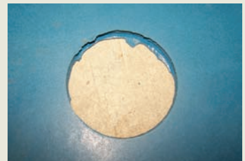
Fig 9. Puncture hole and fragments - polyurethane
