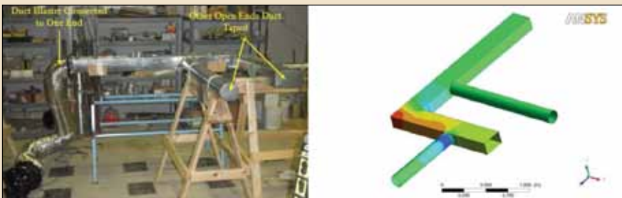
Fig.3 Leak Test using Duct Blaster and Lining using a bladder system
